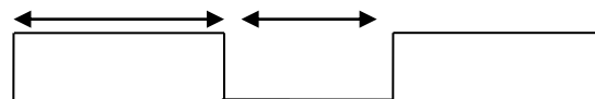
Red LED display pattern next to the connector in the event of an error
